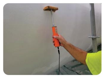
After applying a total overall average DFT of 10.9 mils (one coat of epoxy and two coats of polyurethane), the crew took various measurements throughout, including for thickness.
